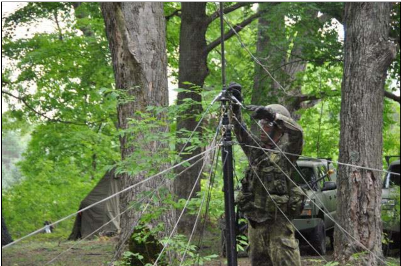
A soldier on the Development Period 1 (DP1) training works to set up a large antenna. The antenna is an integral piece of equipment, allowing a signal detachment to operate in the field. This is a tricky task, as the antenna reaches high into the trees, and must be properly balanced, levelled and secured.
