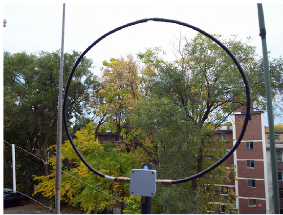
Home built Magnetic Loop Antenna.
