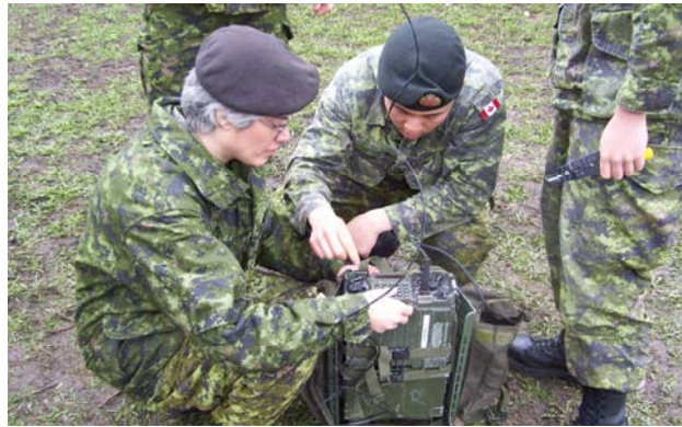
Sapper Moon (right) of 32 CER and Sgt Taylor-Baptiste (left) of 25 Svc Bn program the 522 Net radio.
